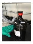
**Causes:** Failure to properly mitigate the hazard presented by volatile chemicals. The bottle was leaking inside the secondary containment.
